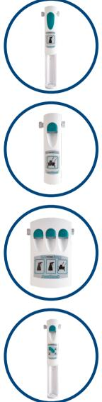
With the push-button operation you automatically dilute chemical concentrates, e.g. for sprayers, buckets, wash basins, scrubbersuction machines and container foam devices. The concentration can be set by changing the individual nozzles/tips. At the touch of the green button, the chemical is drawn into the water stream and mixed with the water. Available in four versions that produce either one, two, three or four different cleaning or disinfecting solutions.
