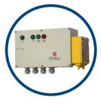
The DSP 9805-II dosing unit has been specially developed for use with crate washers, pack washers and bottle washers. With a delivery rate of 833 ml/min, even large tank contents can be effortlessly brought up to the target concentration when refilling with fresh water. During washing operation, the concentration of the cleaning agent in the washing tank can be continuously and consistently maintained at the desired target concentration in the washing solution, depending on the conductivity.
