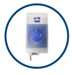
The peristaltic pumps Compact R and Compact K are suitable for continuous dosing of a pre-set quantity (e.g. cleaner). The delivery rate is adjusted via a potentiometer inside the pump. The pumps of the Compact series have a good price-performance ratio. The scope of delivery includes the necessary accessories such as tank inlet connection, container suction and supply hoses.
